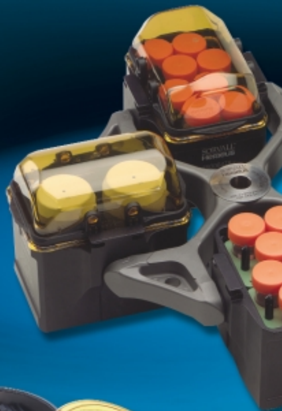
Godet DoubleSpin™ contenant 8 microplaques standard
